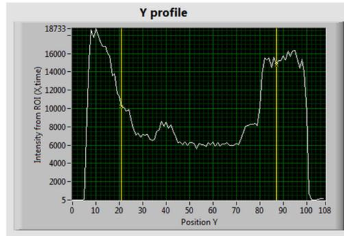
**Figure 3** Example of a one dimensional beam profile for the vertical axis with ROI selection
