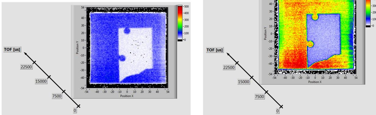
**Figure 6** Two positions of the Two Dimensional Beam Profiler Mode with Time of Flight. Figure left shows beam profile in [0-7500  $\mu\text{s}$ ] range; figure right shows the same in the [7500-15000  $\mu\text{s}$ ] range
