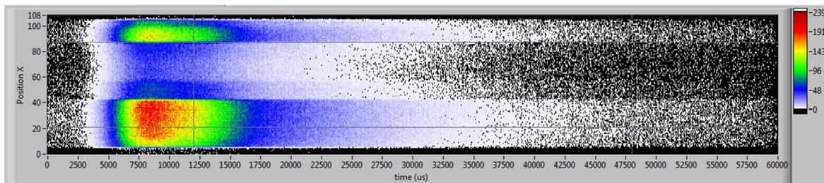
**Figure 4** One dimensional beam profile with Time-of-Flight using the X/horizontal axis
